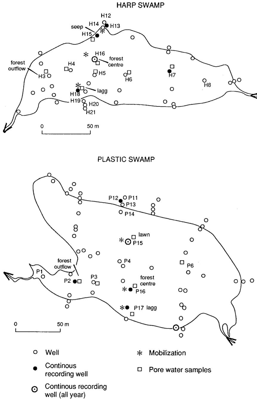
Figure 1. Plastic and HARP swamps showing the location of groundwater wells, piezometers for collecting pore water chemistry, and hollow sites for peat mobilization studies.
