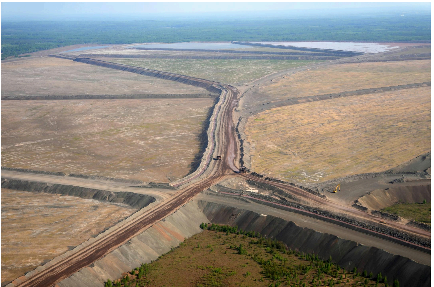
Minntac's tailings basin contains many internal dikes and cells. It's the biggest basin on the Iron Range, covering more than 13 square miles. (Anthony Soufflé/The Minnesota Star Tribune)
