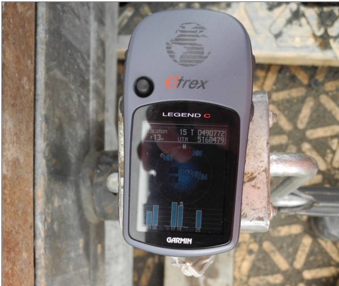
Figure 12.5: Handheld GPS Proximal to Drill Rig (Drill hole 22TK0412 Illustrated, at Final Survey Coordinates 490,774 East, and 5,168,481 North)
