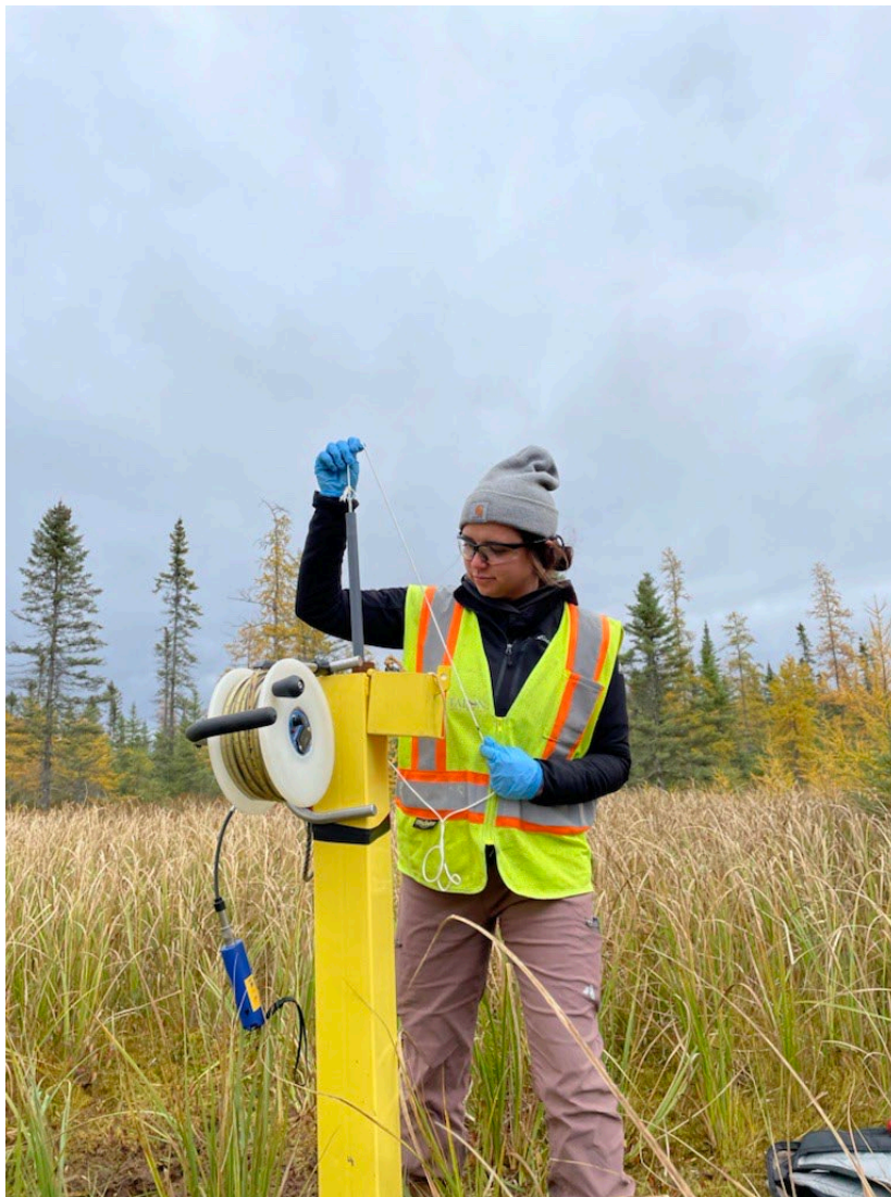
Figure 20.1:Talon Conducting a Slug Test at Tamarack
