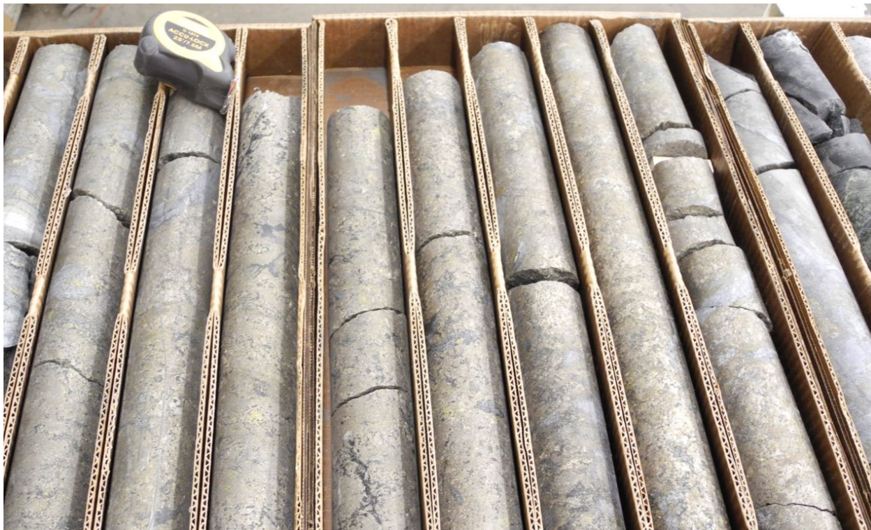
Figure 12.10: Example of High-Grade Drill Core From the Base of the CGO West Mineral Domain.
