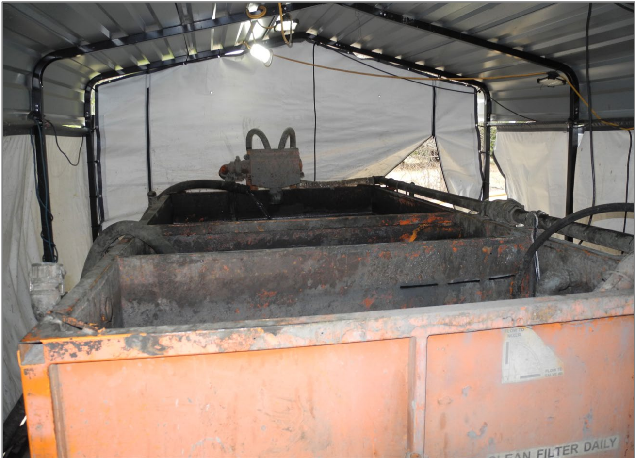
Figure 12.9: Drill Cuttings Are Captured into Bins for Later Disposal.
