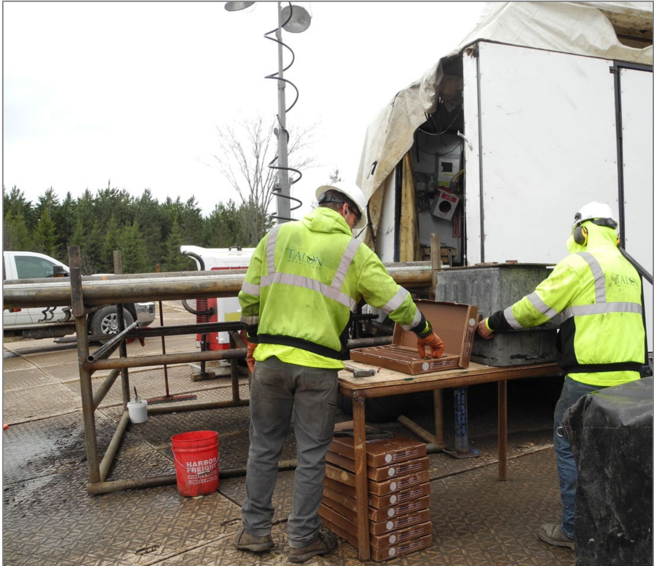
Figure 12.7: Drill Crew Placing Drill Core in Boxes, and Placing Black Bin over Another Box for Digital Photography
