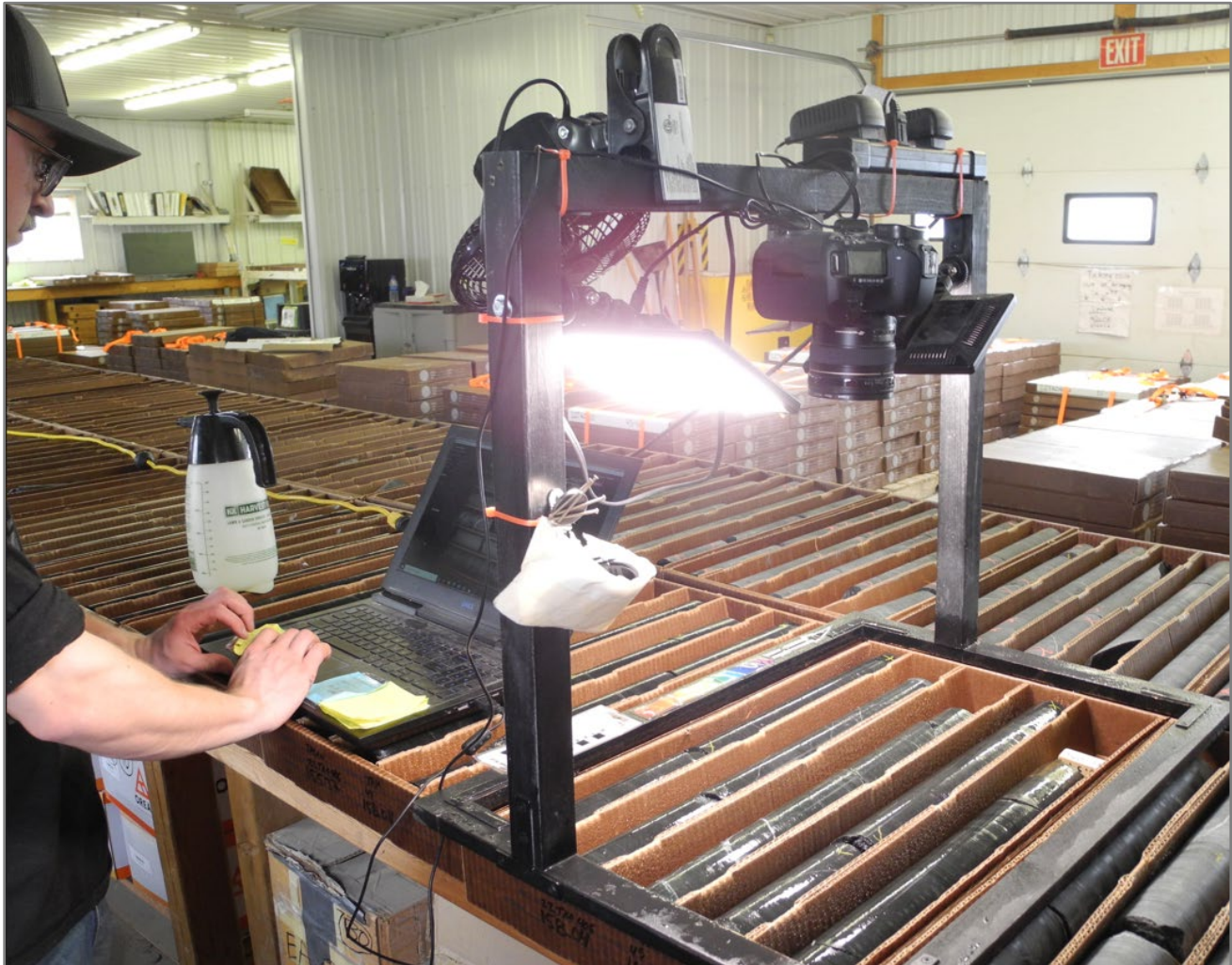
Figure 12.12: Geotechnical Logging of The Drill Core and Bench Photography
