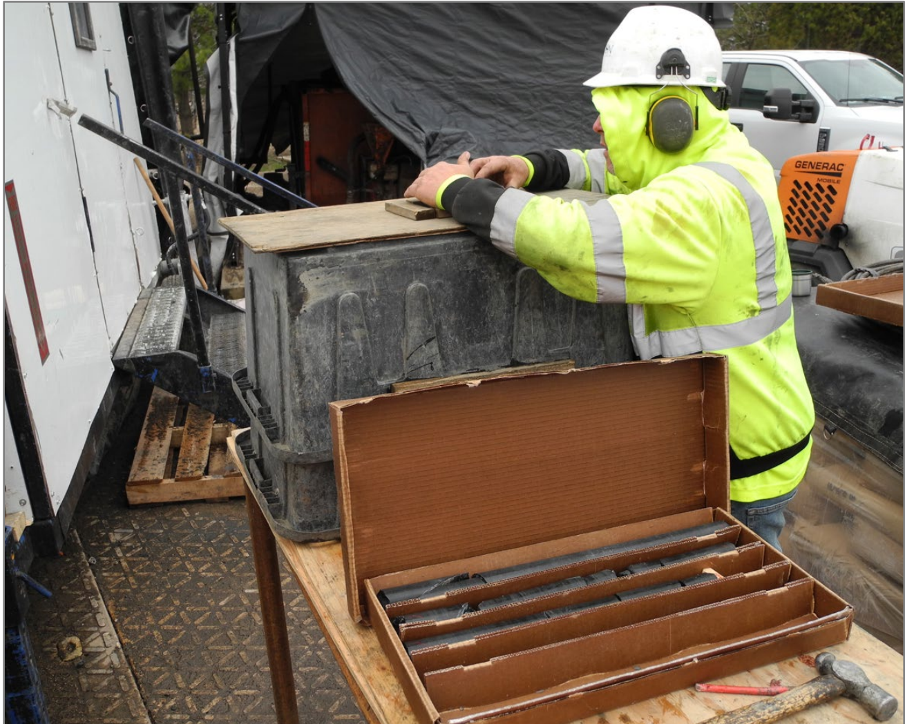
Figure 12.8: Digital Photography of Core in Box Beneath the Black Bin Apparatus, with Drill Crew Sending Photograph via Commercial Cellular Network to a Talon Server.
