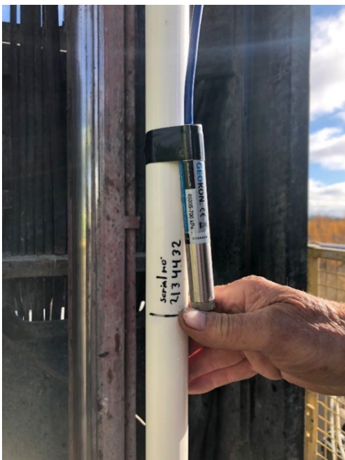
Figure 20.3: Talon installing a Vibrating Wire Piezometer in the Quaternary Deposits at Tamarack
