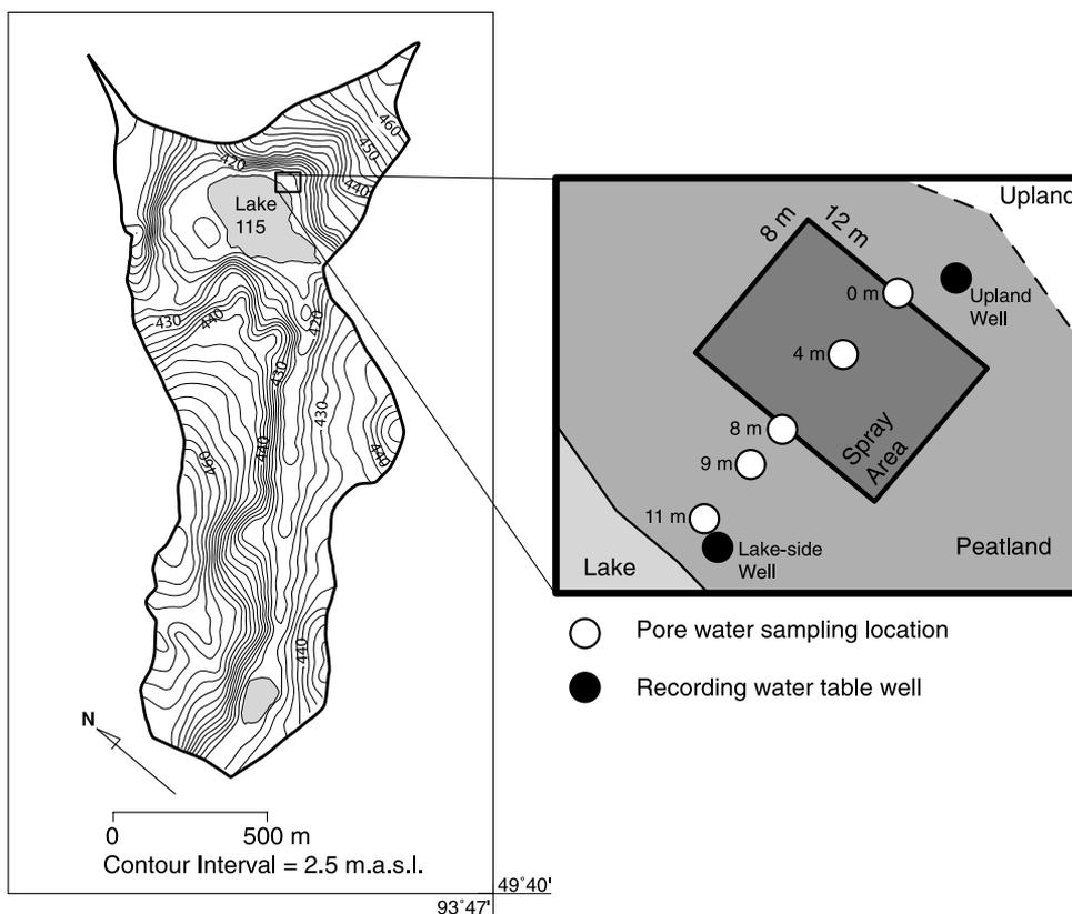
**Figure 1.** Topographic map of the experimental watershed. The location of the study plot and the instrumentation are presented on the inset map.
