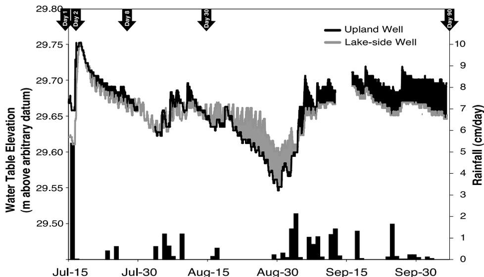
**Figure 2.** Rainfall and water table elevation at the upland (black) and lake (gray) ends of the experimental plot transect for the study period. The normal direction of flow is toward the lake (black line over gray). Flow is reversed from the lake toward the upland during a period of low rainfall (gray line over black). Sampling times are indicated by the arrows at the top.
